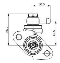
**INLET TYPE 'D'** SELECT MASTER CYLINDER WITH INLET TYPE 'B', PLUS INLET ADAPTER KIT PART NUMBER CP2623-41.
