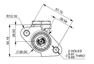
**PUSHROD LEGNTH** 70.56 120 26.60 THREAD LENGTH **IMPORTANT** FITTING OF NUT OF CLEVIS TO FULL EXTENT OF THREAD MAY RESTRICT PISOTN TRAVEL. 50 28. 4.00° PUSHROD ANGULARITY NOT TO EXCEED 4° INC INLET ADAPTER 11.74
