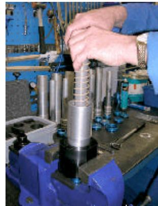
3. Once the Bearing housing is unscrewed completely from the Body, the Air Jack Piston Assembly can be withdrawn from the Body in one piece. **(See Fig 2.)**
